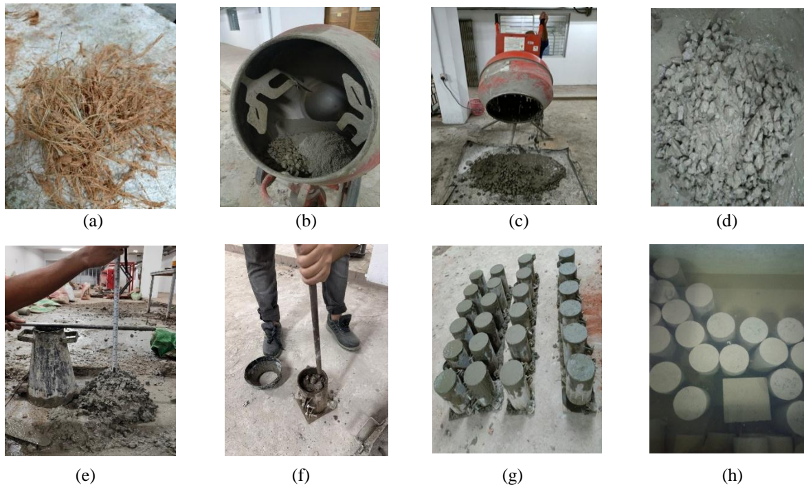
Figure 4: (a) Coconut Fiber, (b) Mixing dry materials, (c) Concrete Mixing Machine, (d) Freshly Poured Concrete, (e) Slump Test, (f) Tamping, (g) Concrete Cylinder Making, (h) Curing
