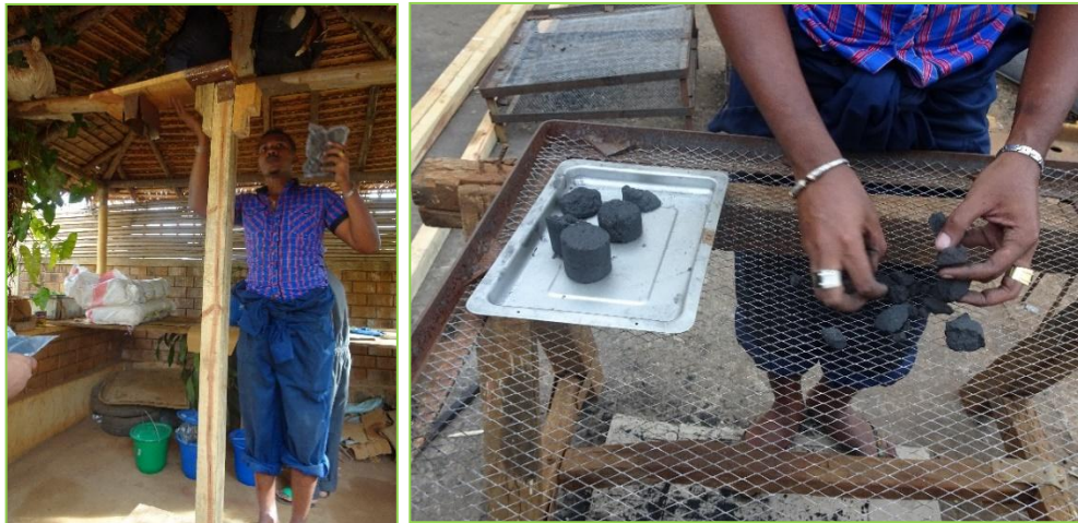
Figure2: Principle of the Briquette Shock Resistance Test
