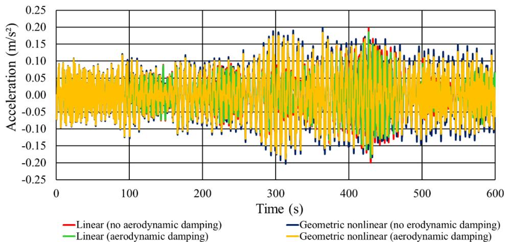
Figure 7: Geometric nonlinearity and aerodynamic damping effects (accelerations)  $V_0 = 126 \text{ km/h}$
