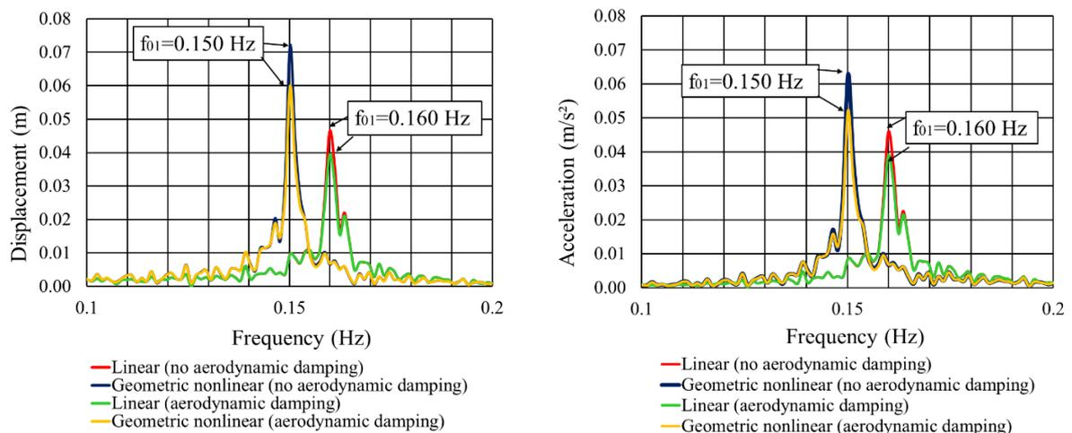
Figure 8: Dynamic response (frequency domain): displacements and accelerations  $V_0 = 126 \text{ km/h}$
