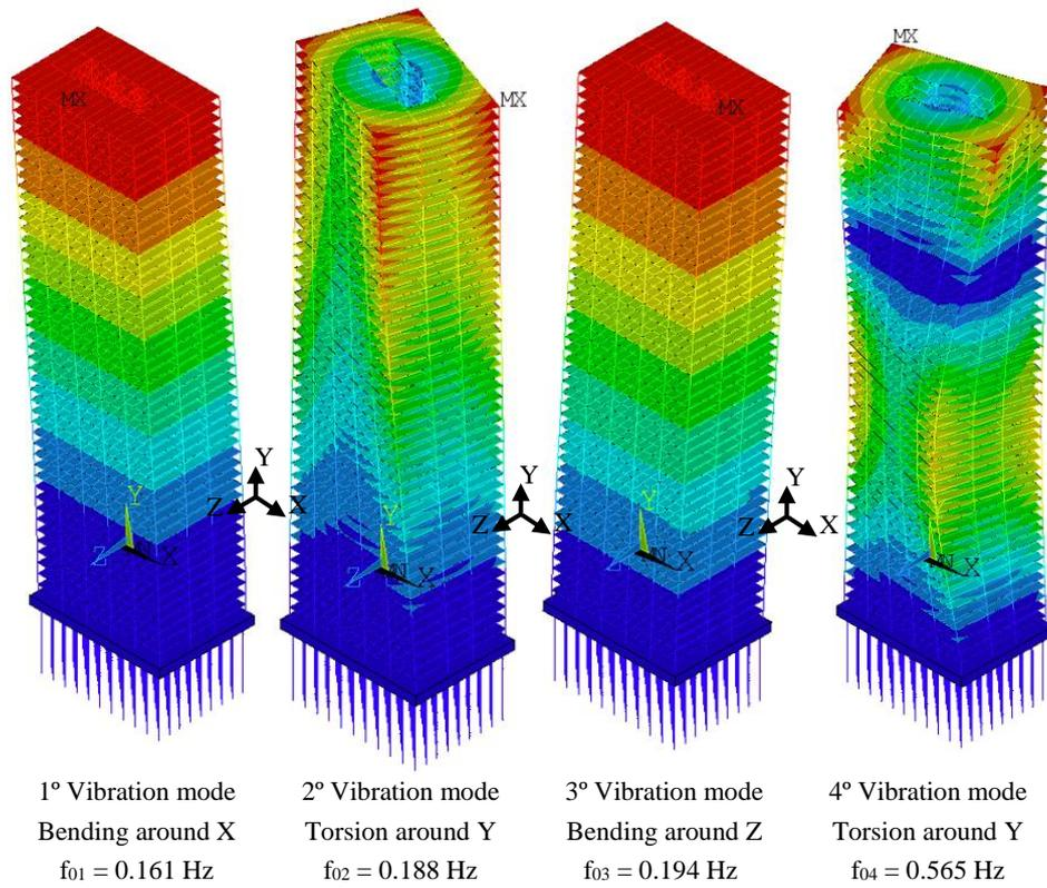
**Figure 5: Vibration modes of the analysed steel-concrete composite building**
