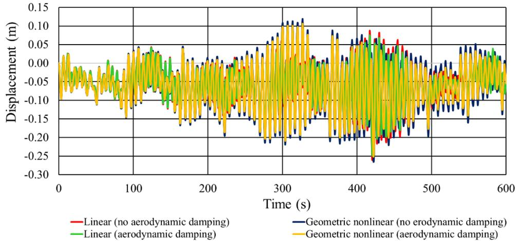
Figure 6: Geometric nonlinearity and aerodynamic damping effects (displacements)  $V_0 = 126 \text{ km/h}$
