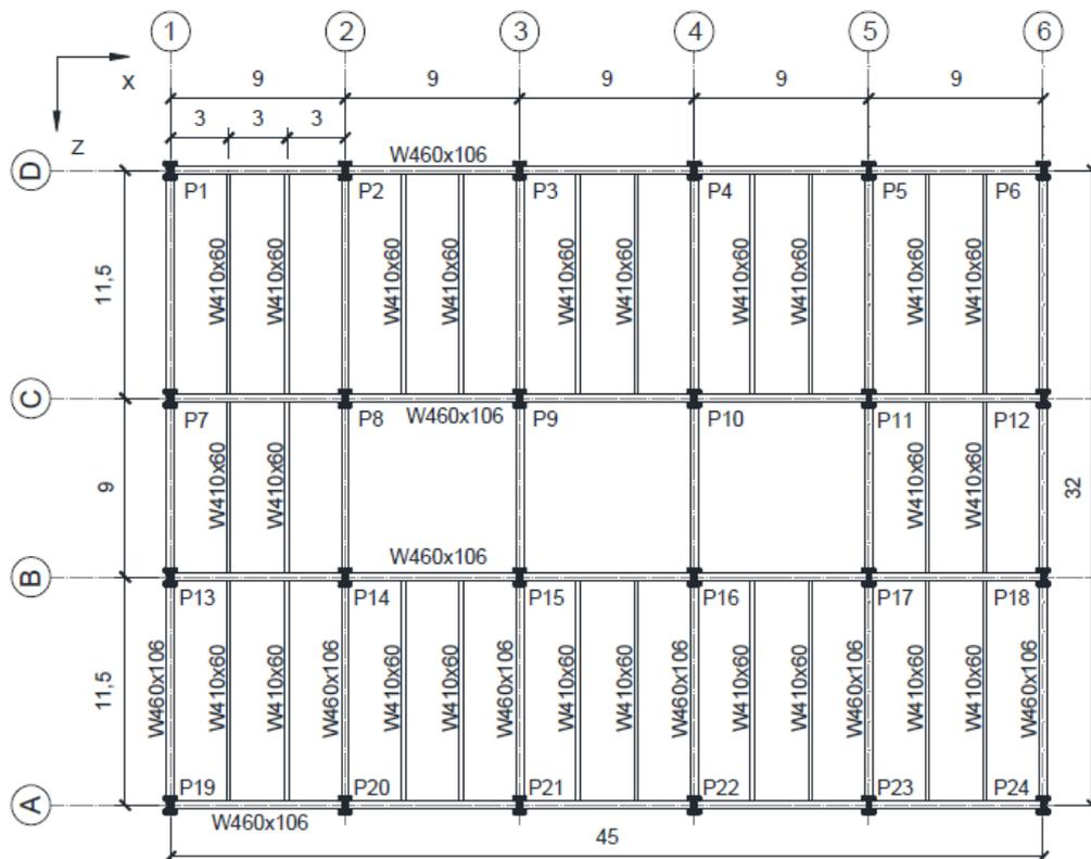
Figure 3: Structural design of the steel-concrete composite building.
