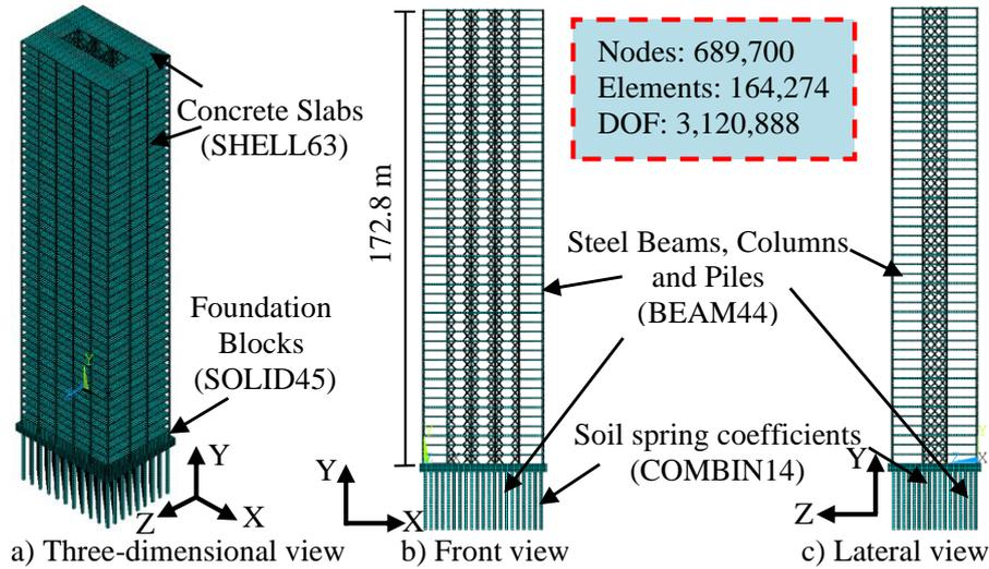
**Figure 4: Finite element model of the steel-concrete composite building**
