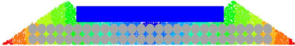
Figure 6: Layout Diagram of Measurement Circles at the Ballast Bed Monitoring Points
