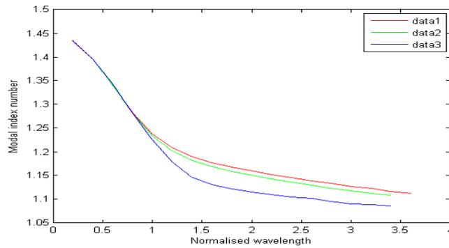
Fig. 5 Modal index number versus normalized wavelength curve. (Data1, data2, and data3 represent the structures in Fig 1(b), 2(b) and 3(b) respectively)
