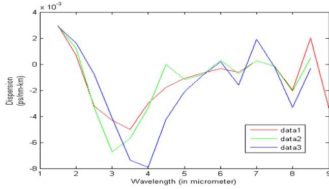
Fig. 5 The curve between dispersion and wavelength of all the proposed structure in this paper. (Data1, data2 and data3 represents the structure of Fig. 1(b), 2(b) and 3(b) respectively).
