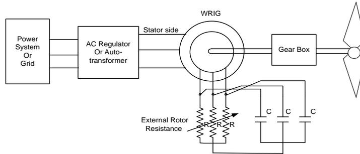
Fig. 14 : Circuit topology of the proposed scheme with capacitor
