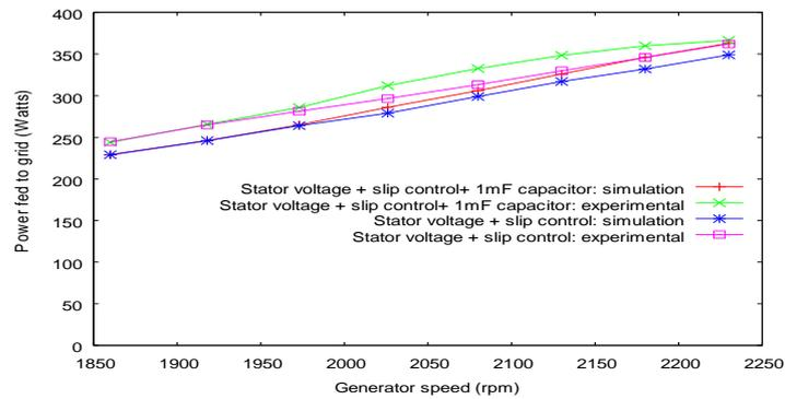
Fig. 18: Power fed into grid for different speed
