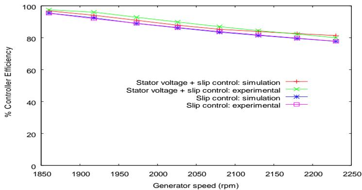
**Fig. 9: Controller efficiency for different speed**
