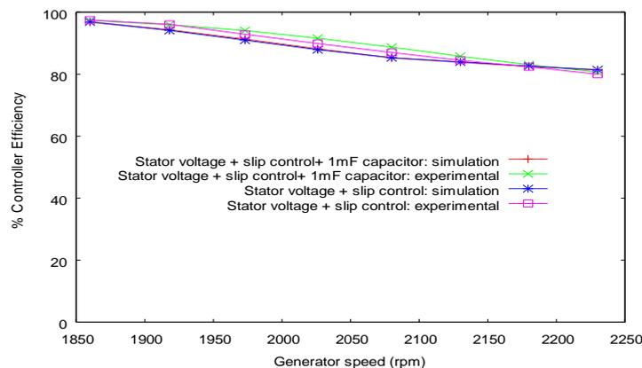
Fig. 15: Controller efficiency for different speed
