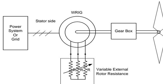
Fig. 1 : Slip power control scheme of a wound rotor induction generator
