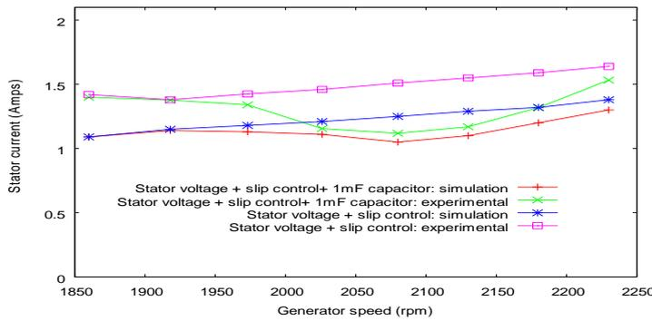
Fig. 17: Stator current for different speed
