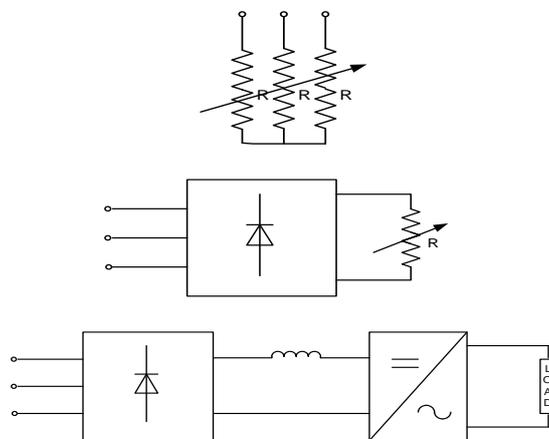
Fig. 5: Circuit topologies of the slip power controller circuit
