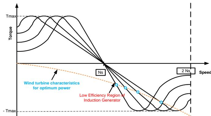
Fig. 2: Characteristics of a WRIG with rotor resistance control
