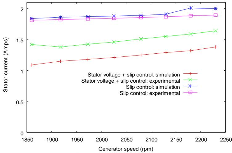
Fig. 11: Stator current for different speed
