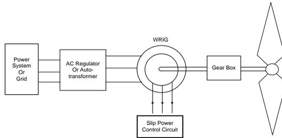
Fig. 3: Circuit topology of the proposed scheme
