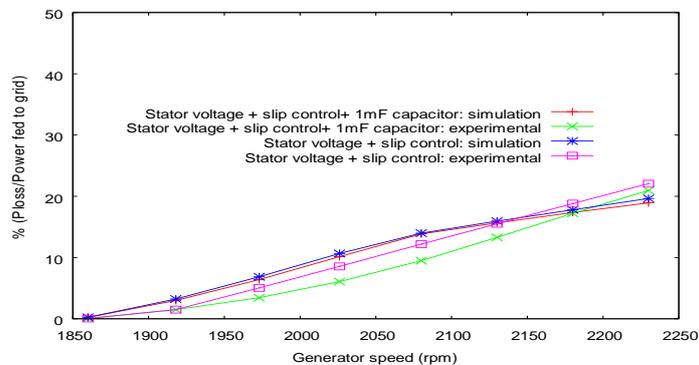
Fig. 19: Percentage of power loss in the external resistor with respect to power fed to grid for different speed
