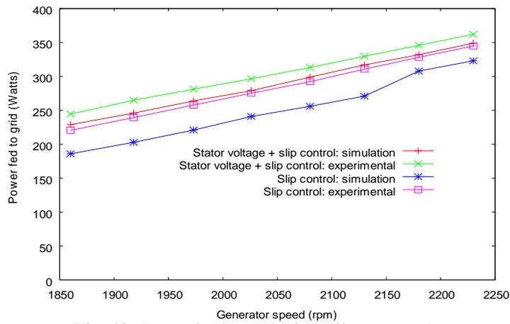
Fig. 12: Power fed into grid for different speed
