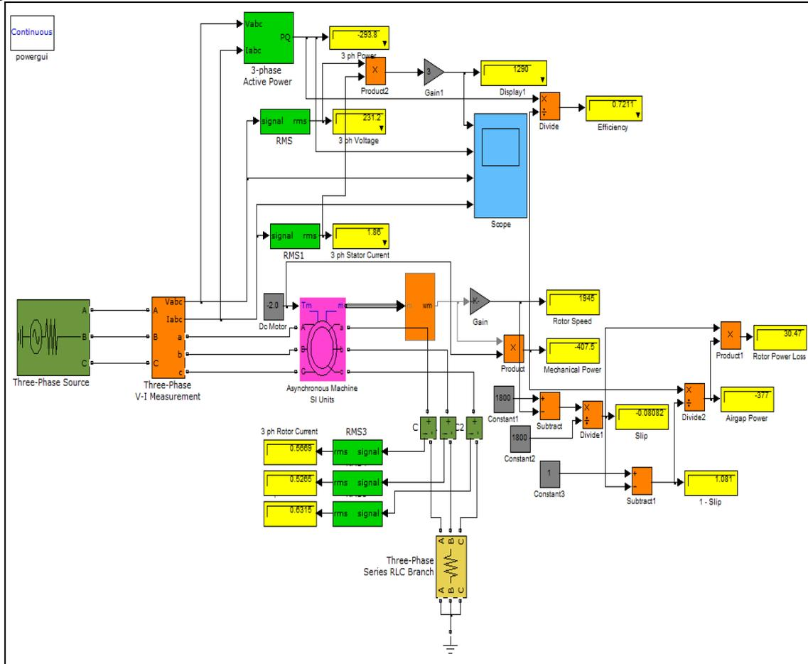
Fig. 6: MATLAB Simulation model of the proposed system feeding power into the grid.
