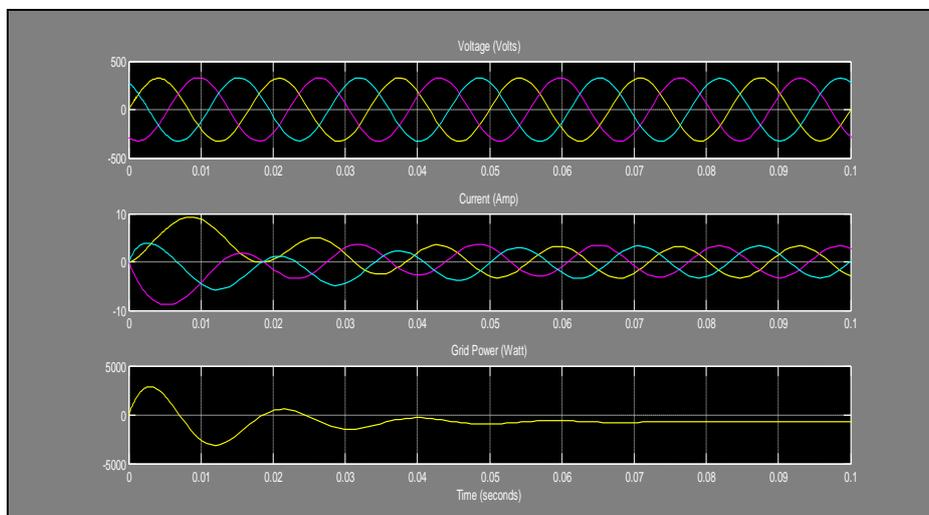
Fig. 7: Waveform showing stator voltage, stator current and power fed to grid
