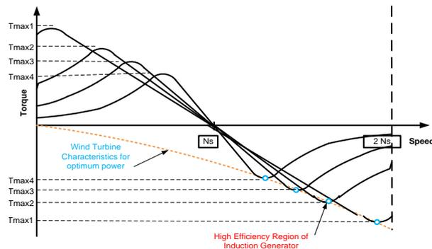
Fig. 4: Characteristics of a WRIG with rotor resistance as well as stator voltage control
