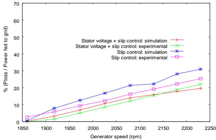
Fig. 13: Percentage of power loss in the external resistor with respect to power fed to grid for different speed
