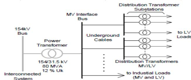
Fig.2 A typical part of radially operated distribution system (Gray color indicates the transmission system, black color indicates the distribution system)
