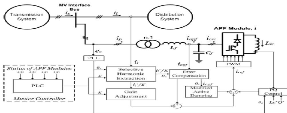
**Fig4.** Block diagram representation of the control system for each APF module
