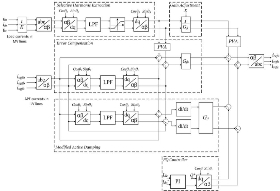
Fig.5 Block diagram representation of the reference current generation circuit
