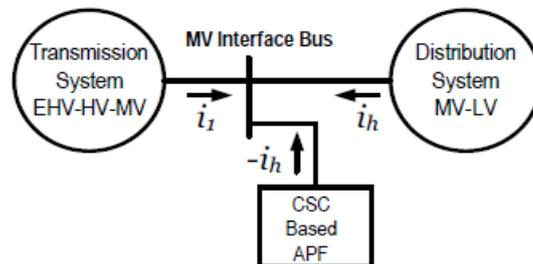
Fig.3 CSC based APF system connected to the MV interface bus
