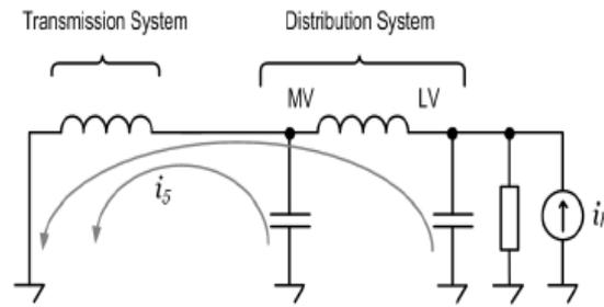
Fig.1 Illustration of parallel resonance
