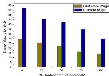
Figure 4: Energy Absorption at First Crack and Ultimate stage
