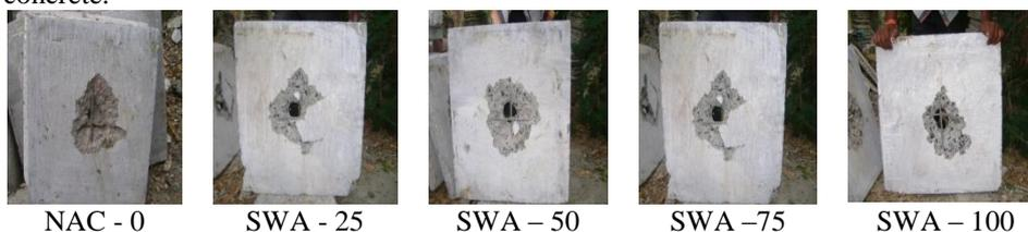
Figure.5: Tested slab specimens
