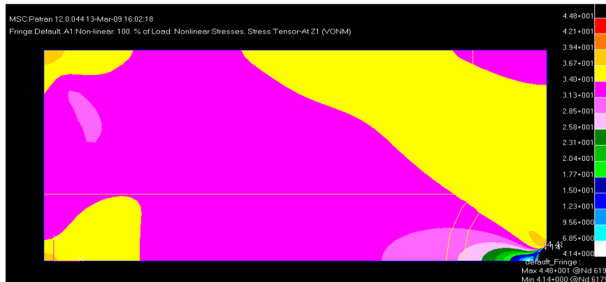
Fig.7: Plastic FEA result of elliptical cut out for a=10, b=5 (Al 2024 T-3)
